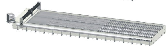
160X-3 X-Y切割行程: 14224 mm x 4064 mm
