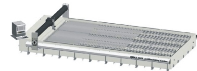
160X X-Y切割行程: 8128 mm x 4064 mm
